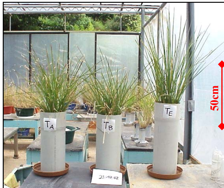
Figure 16: Vetiver plants in contaminated soil (Treatment A [T A ]: medium fertilizer level, Treatment B [T B ]: high fertilizer level) and in uncontaminated soil (Treatment E [T E ]: low fertilizer level) after 6 months of growing. The height of pots differ a little, but they contain the same quantity of soil medium in the same density. (Brandt, 23.10.2002)
