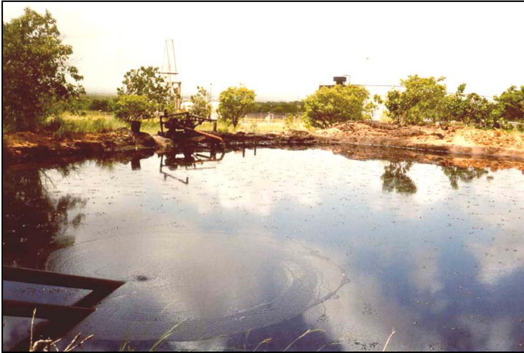
Figure 2: Reserve pits of drilling wastes in El Tigre, Anzoátegui State, Venezuela (Brandt, 08.09.2001)
