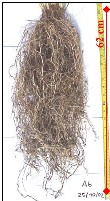
Figure 22: Vetiver roots in contaminated soil after 6 months of growing (Treatment A: medium fertilizer level). Root length: 62 cm. (Brandt, 25.10.2002)
